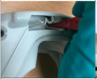
10. Once the assembly is seated while holding a downward pressures with the tweezers, turn the lever clockwise until it is firmly positioned under the locking nub.
