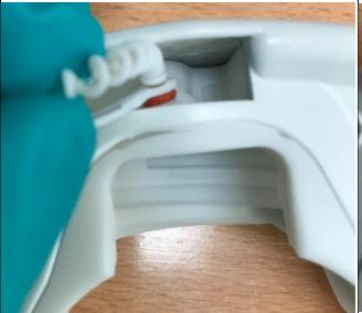
7. Carefully slide the assembly into the unit with the lever arm pointing out.
