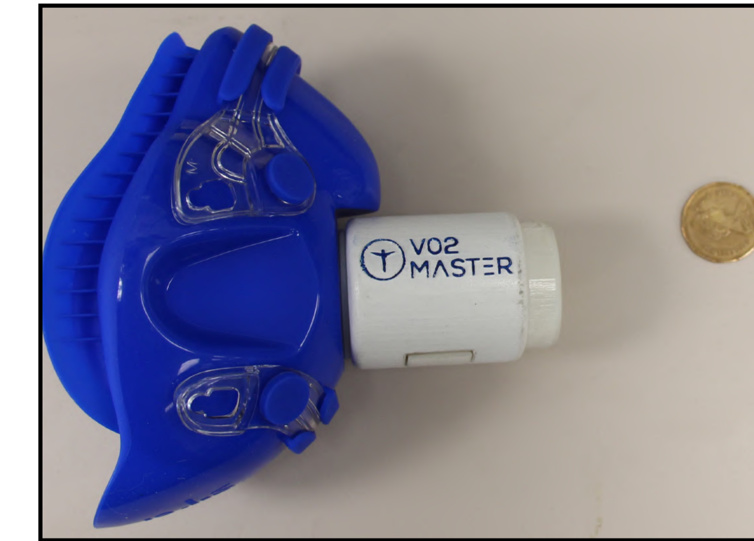
Pic2: VO2master Beta-Prototype V2, entirely face worn VO2 analyzer
